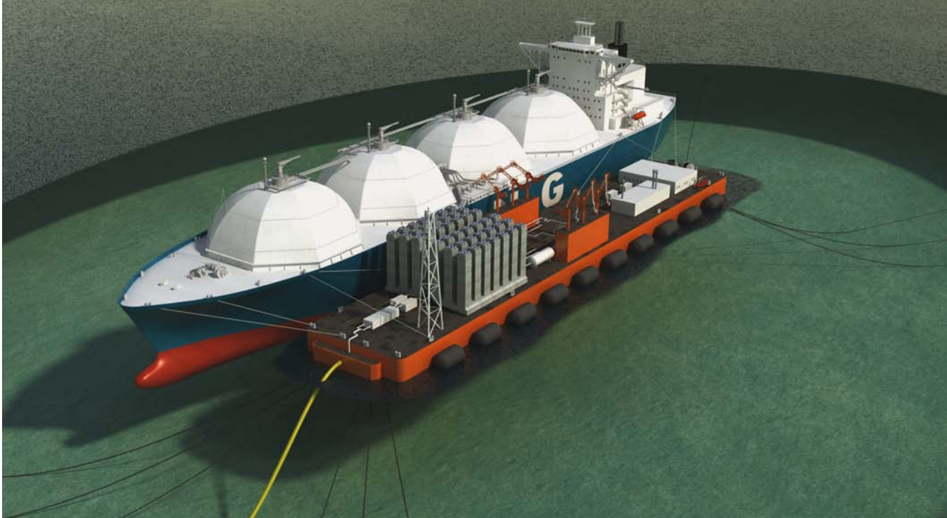
Torp's barge-mounted EasyLNG concept is a regasification solution for shallow water and benign environments
